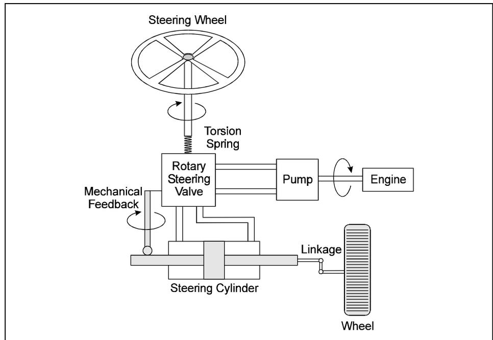
In the design stage, it is in the engineer's interest to know the proportionality of power assistance to the steering wheel torque. Normally, the power assistance gain is characterized by the static pressure drop across the rotary steering valve versus the opening area (restriction) of the valve. The pressure gain curve can be tuned to provide the optimum assistance needed for any driving condition.
